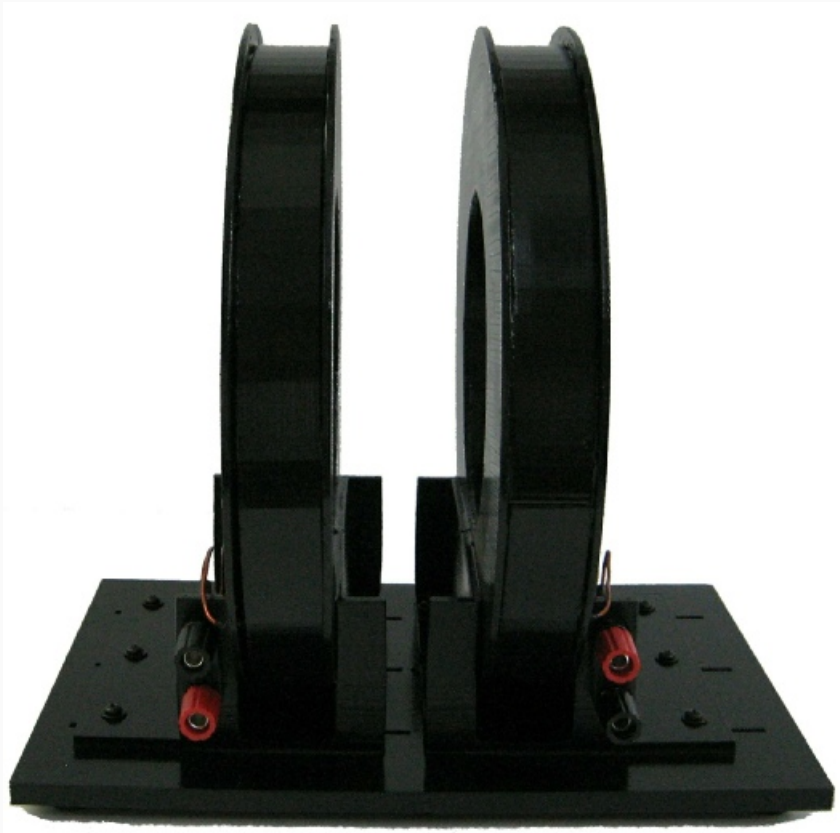
207mm diameter Helmholtz coil pair for generating 20mT
