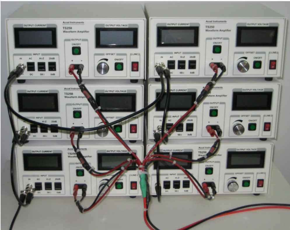
Six TS250-2 amplifier connected together using a custom-made harness to obtain 32A peak-to-peak current.
