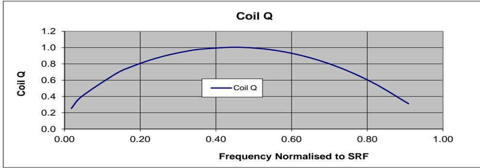
Figure 3.1 Coil Q with the effects of SRF
